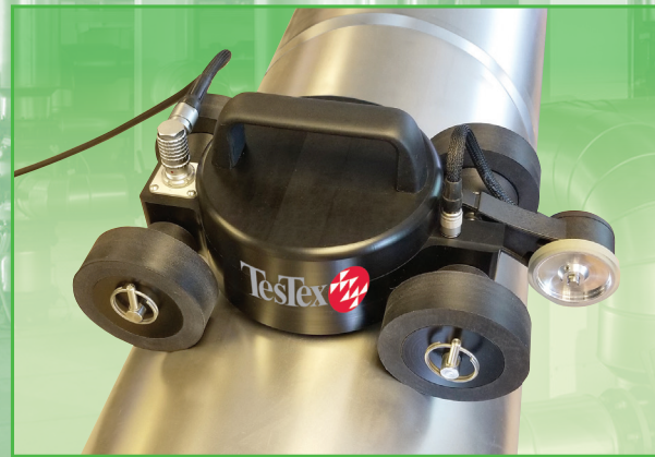
OSET Scanner Performing a Circumferential Overlap Scan
