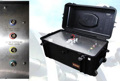
Control board delivers registered data packages to the software for further visualization, and test reports creation.
