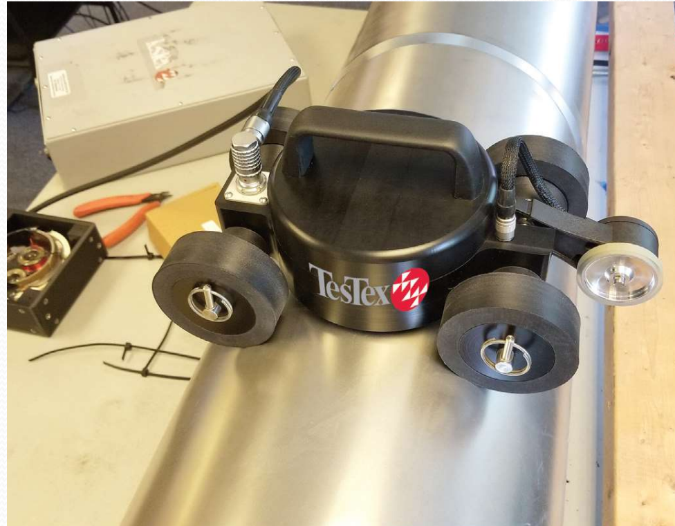
OSET Scanner performing a circumferential overlap scan
