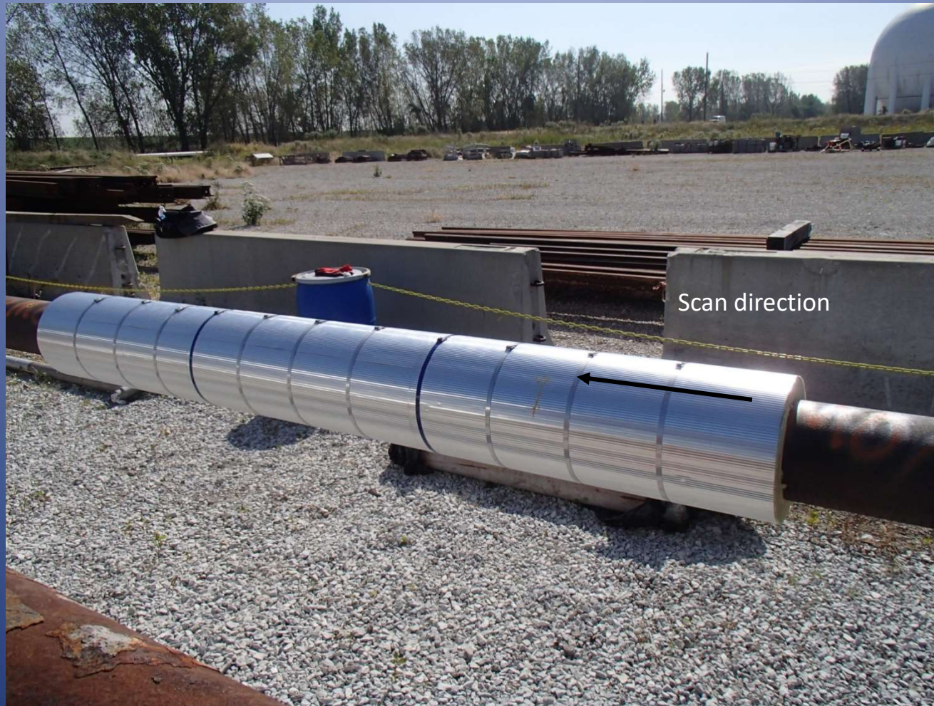
Picture of a pipe scanned as part of a test of the OSET technology. This was a pipe with natural corrosion that was removed from a process line.
